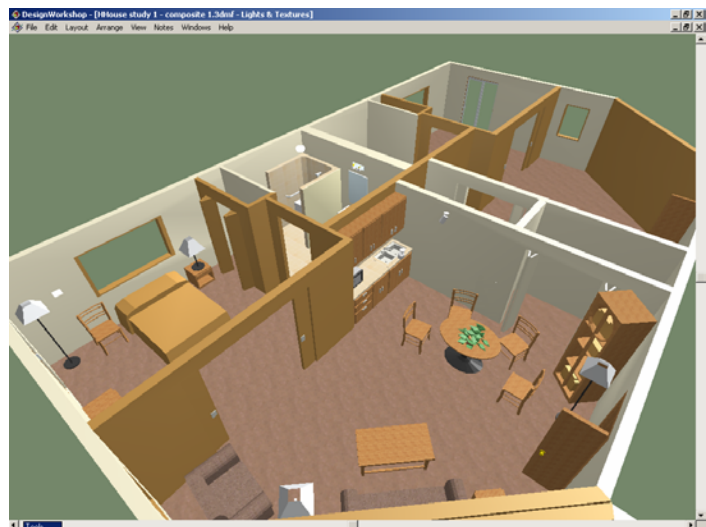
Figure 3. An early attempt to represent some of the emerging specifications for the apartment units. Note the double pocket doors connecting the bedroom with the living area, the small kitchenette with sink and microwave, and the “roll-in” shower.
